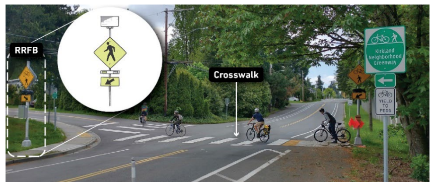
Example of a rectangular rapid-flashing beacon (RRFB), a pedestrian-activated device that can be placed at crosswalks to increase compliance of vehicles yielding to pedestrians. They have two rectangular-shaped yellow indications, each with an LED-array-based light source that flash with high frequency when activated. When the lights are activated by pedestrians, drivers should stop like a stop sign.
